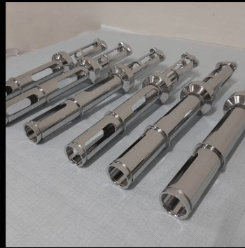
ELECTROLYTIC PLASMA POLISHING OF THE PART TO A REFLECTIVE CONDITION
